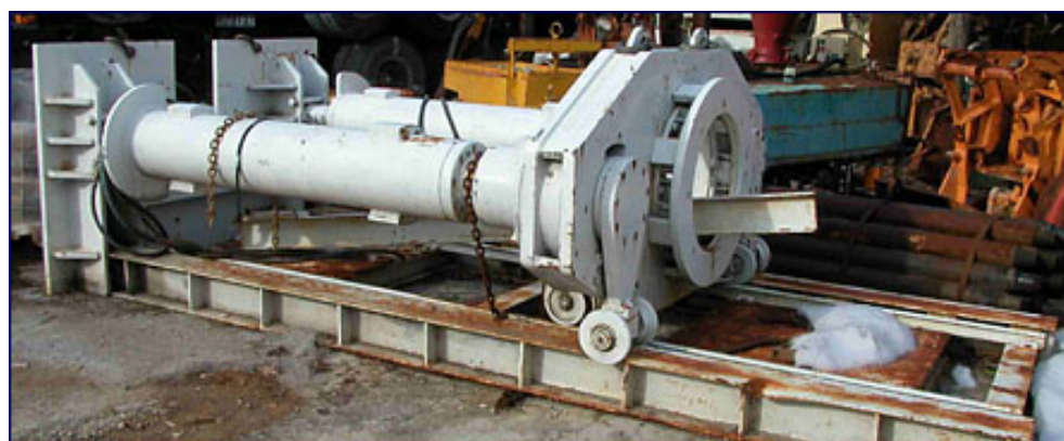
FIGURE 5.3: AN EXAMPLE OF JACKING FRAME (Courtesy of Bradshaw Corp)
