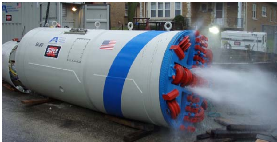
FIGURE 5.1: MICROTUNNEL BORING MACHINE (Courtesy of Akkerman)
