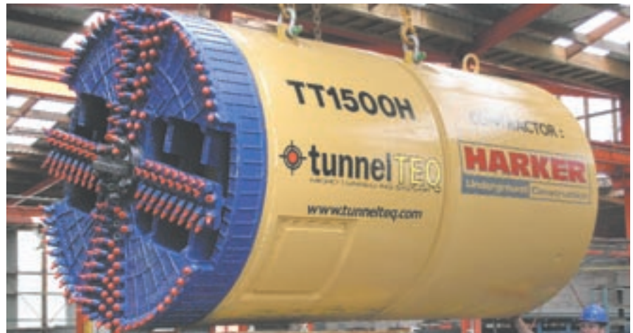
■ 1500NB microtunneller used on Wellington City Storm Water upgrade.
