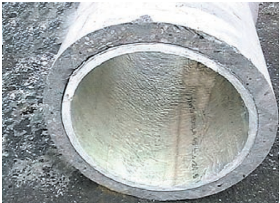
■ 18mm Enviroliner inside a 525mm test pipe.
