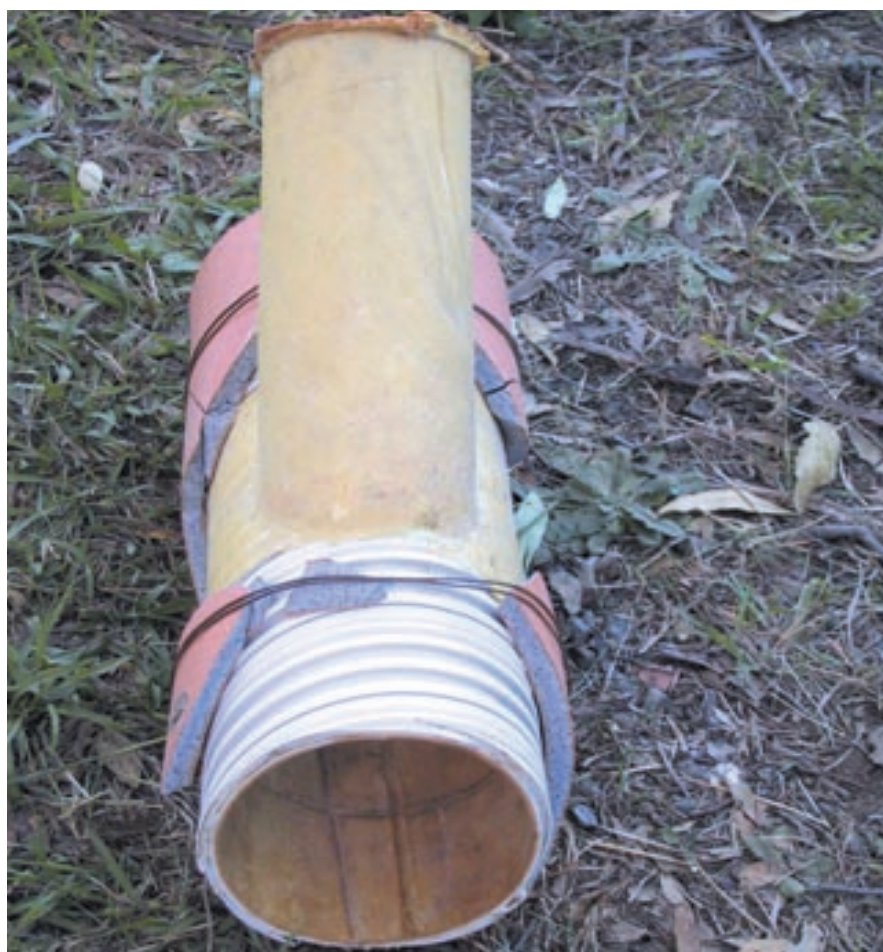
■ Interflow L.C.R. removed from a sewer junction following a trial installation. An effective physical barrier to root infestation has obviously been provided.
