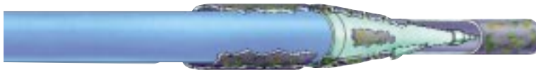
Pipebursting systems use a pneumatic or hydraulic bursting head to break out the old pipe, while simultaneously drawing in a new pipe string
