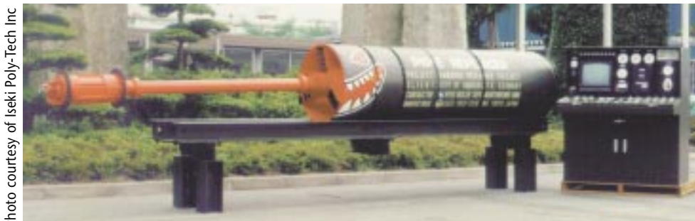
Pipe eating and replacing system with flow-through facility
